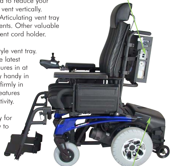
Extra batteries always added under the base.
