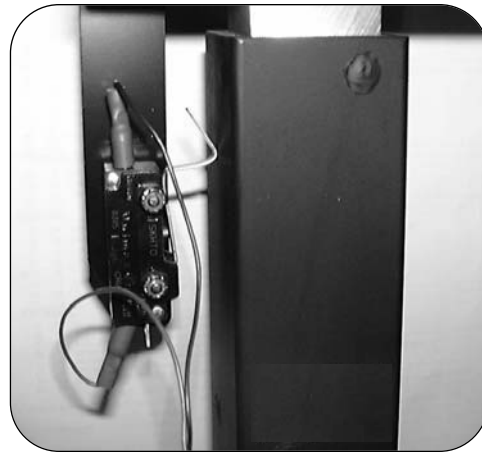
eg. Vertically mounted microswitch on an elevate-only seating system
