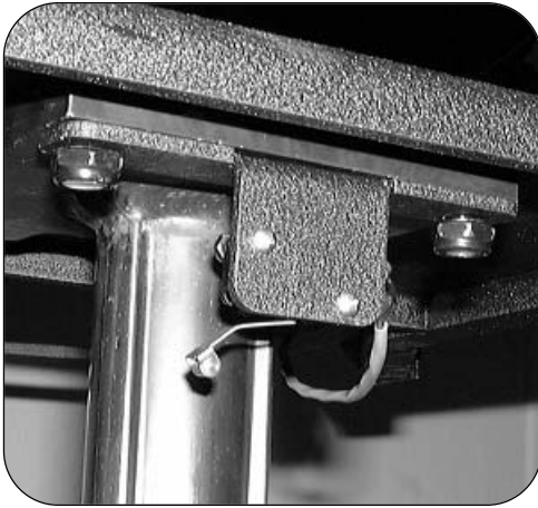
eg. Horizontally mounted microswitch on a PES system with tilt/recline
